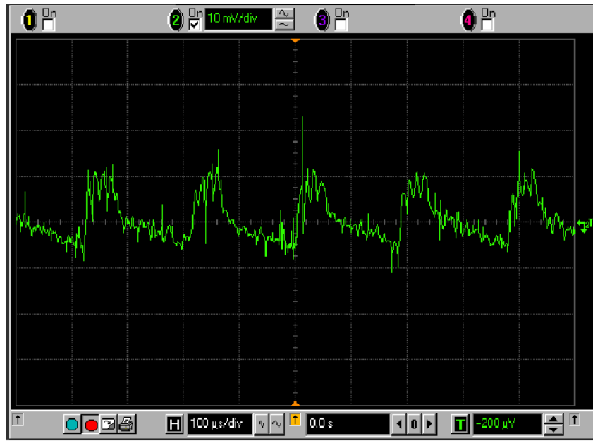
Figure 16. Peak-to-peak ripple, P_{out} = 0.5\text{ W} , Cable length = 30 cm, V_{in} = 230\text{ Vac} .
