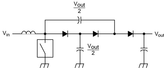
Figure 12. Boost Controller with Increasing Voltage Capability
