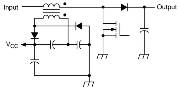
Figure 7. Auxiliary Winding in Boost
