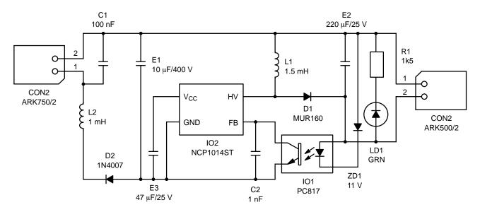
Figure 1. Complete Schematic Diagram of the 12 V/0.2 A Converter
