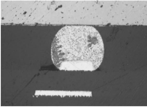
Figure 4. Cross Section of Flip Chip Solder Bump
