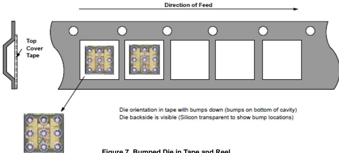
Figure 7. Bumped Die in Tape and Reel
