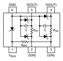
Figure 6. STF202 Device Schematic
