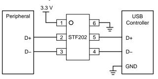
Figure 15. Connection for Low-speed Devices
