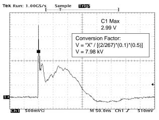
Figure 9b. Real Waveform Sample Taken from ESD Generator
