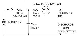
Figure 8. ESD Generator, Simplified Diagram
