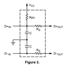
In order to determine if the line is an upstream or downstream line, the USB uses pull up or pull down resistors on the D+ and D– lines, so if a 15 k $\Omega$  pull down resistor is connected on either the D+ or D– line, the port is identified as downstream and in the other hand, if a 1.5 k $\Omega$  pull up resistor is connected on either the D+ or D– line, the port is identified as upstream. Figure 3 illustrates the termination for an upstream USB port.
