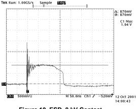
Figure 10. ESD, 8 kV Contact
