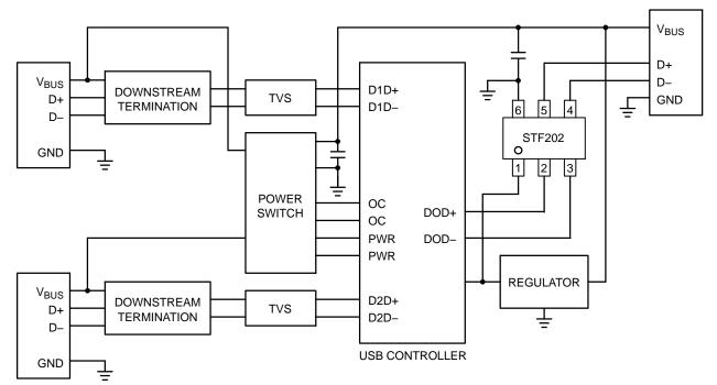
Figure 17. Example of a USB Hub Design
