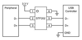
Figure 14. Connection for Full-speed Devices
