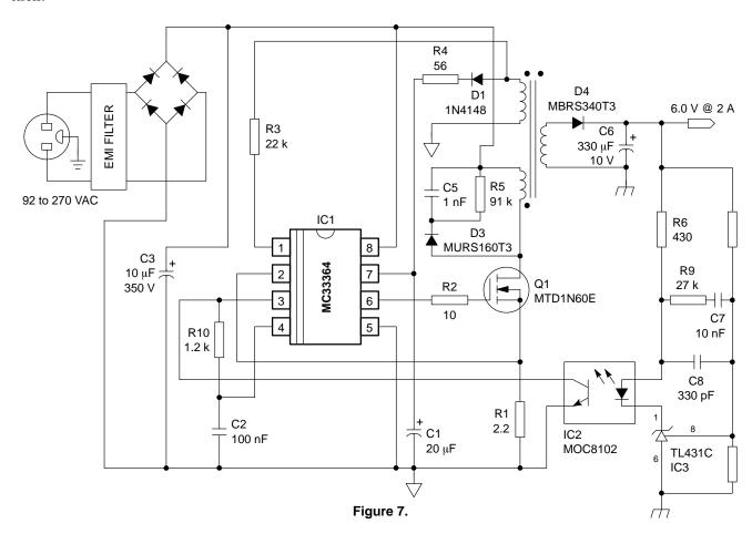
The leakage energy spike is clipped by the R5–C5 network whose second function is to smooth the rising drain voltage, correspondingly limiting the radiated noise. This last feature is unfortunately no longer valid when you use a clipping circuit made of a fast rectifier and a zener diode. The circuit's sensitivity to the noise present on the sense
