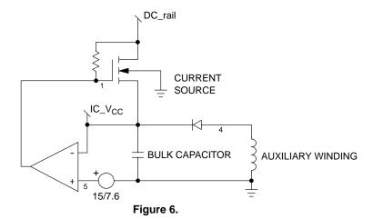
It works as follow: when the mains is first applied to the converter, the MOSFET charges up the bulk capacitor until the voltage on its pins reaches the startup threshold of 15 V. At this time, the MOSFET opens and the circuit operates by itself.
