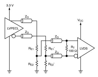
Figure 14. Interfacing 3.3 V LVPECL to LVDS
