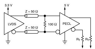
Figure 20. Interfacing LVDS to PECL
