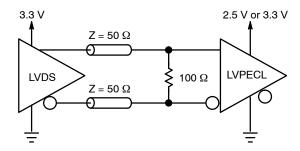
Figure 17. Interfacing LVDS to LVPECL
