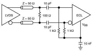
Figure 3. Capacitive Coupling LVDS to ECL Using  $V_{BB}$
