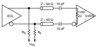
Figure 5. Capacitive Coupling ECL to LVDS
