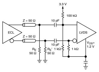
Figure 7. Capacitive Coupling ECL to LVDS Using  $V_{OS}$  Reference Voltage
