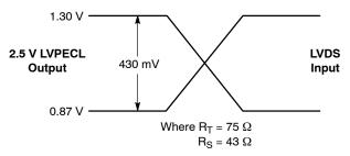
Figure 13. PSPICE Simulation Levels of 2.5V LVPECL to LVDS Interface with Series  $R_S$  Resistor
