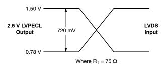
Figure 10. PSPICE Simulation Levels of 2.5V LVPECL to LVDS Interface with Example Resistor Values
