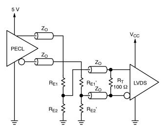
Figure 18. Interfacing 5 V PECL to LVDS
