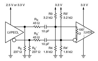
Figure 6. Capacitive Coupling LVPECL to LVDS
