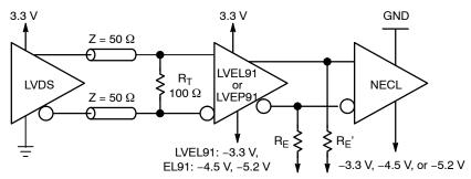
Figure 22. Interfacing from LVDS to NECL
