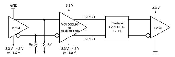
Figure 21. Interfacing from NECL to LVDS
