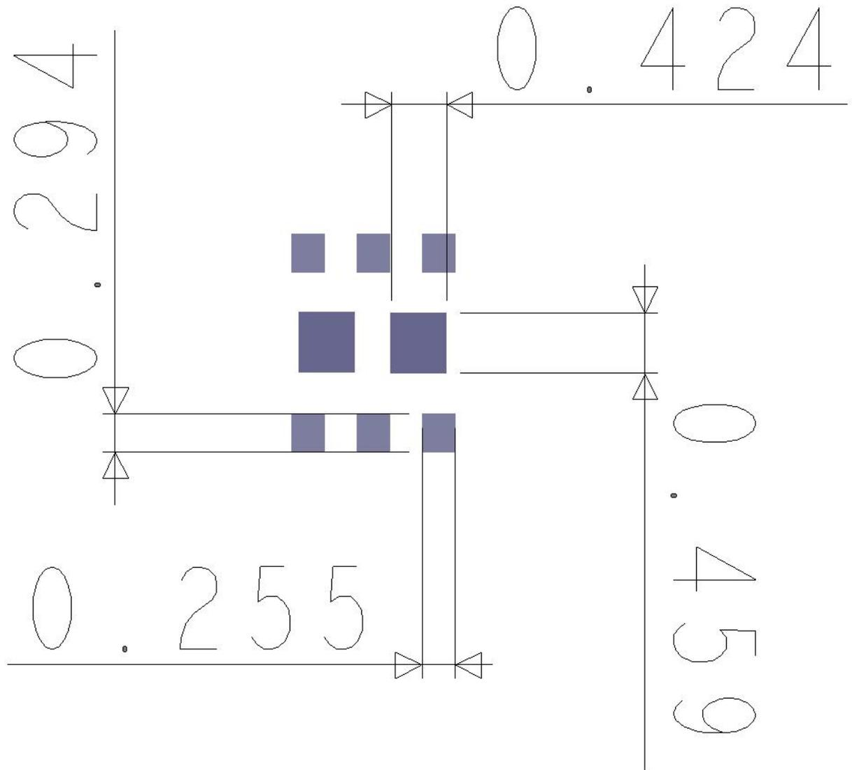
Figure 4. Solder Stencil Opening Recommendations (mm)
