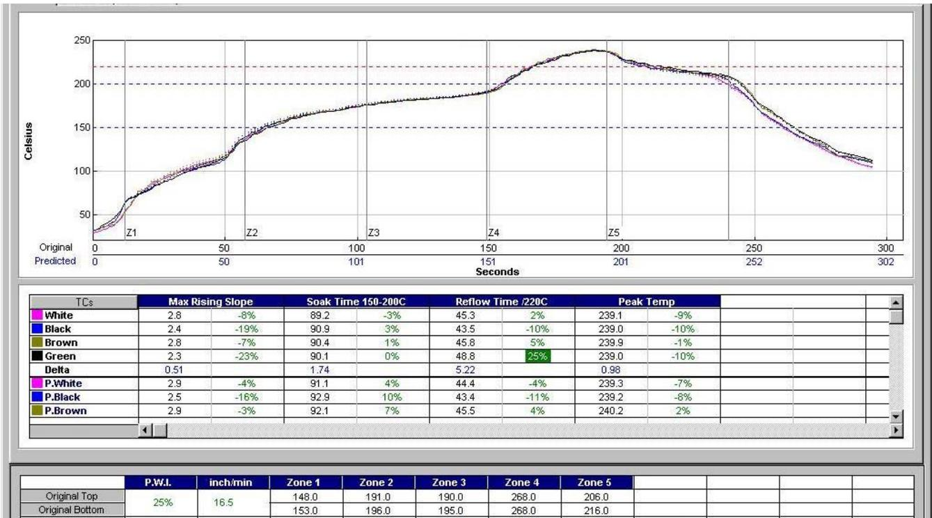
Figure 5. Reflow Profile used for Building Demonstration Boards
