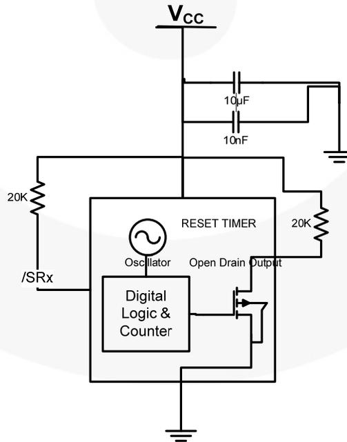
Figure 6. Reset Timer Decoupling and Pull-Up Resistor Reference Schematic (FT8010<sup>(2)</sup> Shown)
