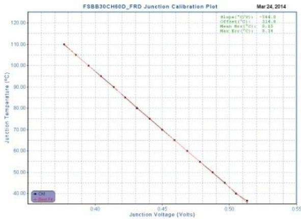
Figure 10. Results of Device Junction Calibration for FRD
