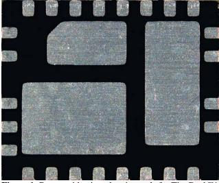
Figure 1: Bottom side view showing pads for TinyBuck<sup>TM</sup>
