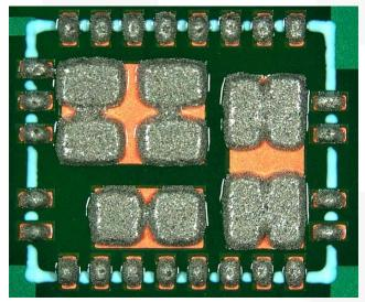
Figure 4: Printed Solder Paste.
