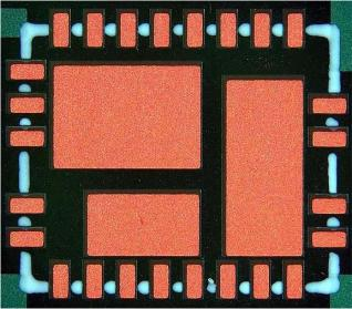
Figure 3: PWB pad showing OSP pad finish.
