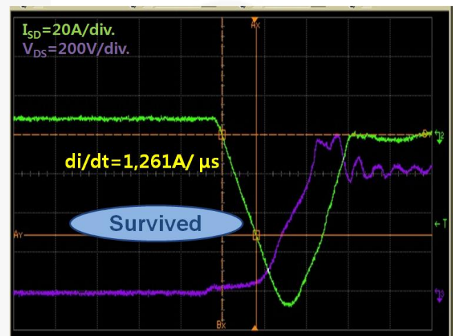
(a) 800 V SuperFET ® II MOSFET Withstanding Waveforms During Body Diode Reverse Recovery
