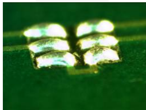
Figure 7. Figure 7-Solder "Bumped" Pads
