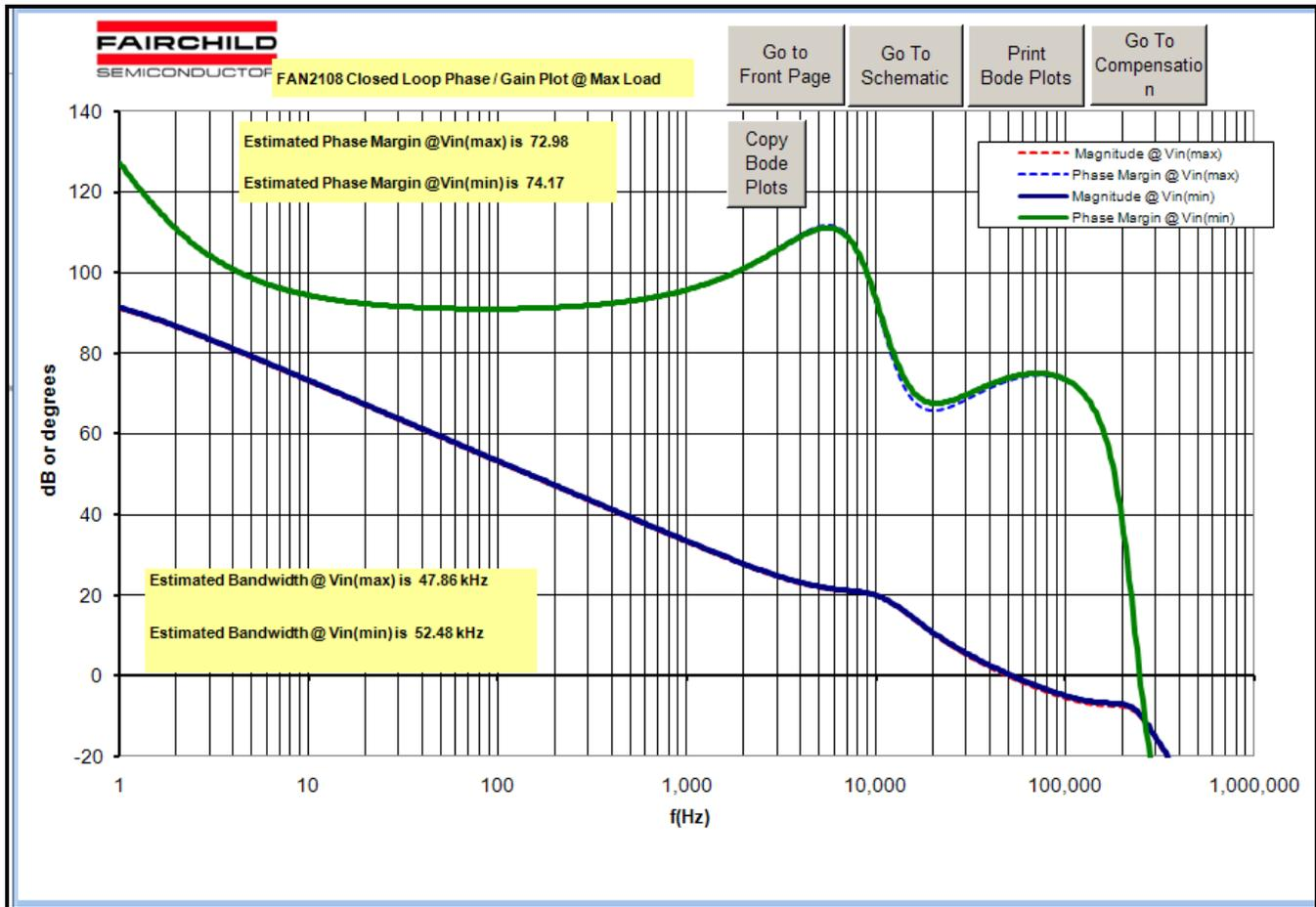
There are text boxes that display the crossover frequency (bandwidth) and the phase margin for this design. Typically, it is a good idea to have greater than  $60^\circ$  of phase margin and bandwidth less than one fifth ( $1/5$ ) of the switching frequency. Each time you return to this page, the new plot is based on the components selected.
