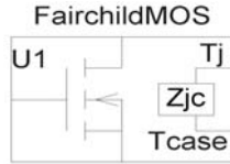
Figure 2 Self-heating MOSFET SPICE symbol
