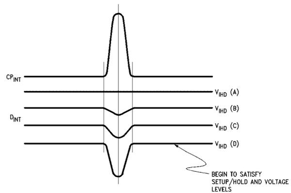
Figure 7. Data Input Level Can Cause Output Errors
