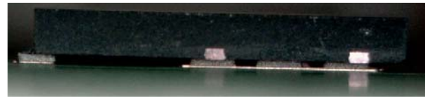
Figure 17. Package Placement Offset, After Reflow Along the Length of the Leads
