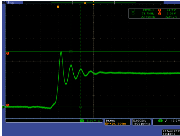
Figure 5. Switch Node Original Ring Waveform
