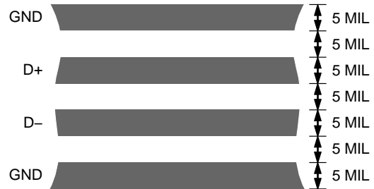
Figure 34. Typical Arrangement of Signal Tracks
