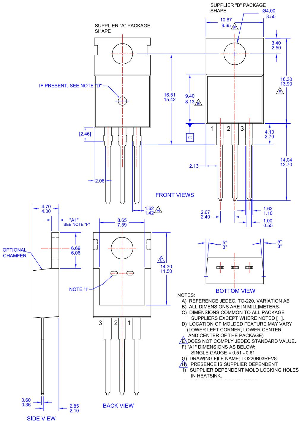
Figure 5. TO-220, MOLDED, 3LEAD, JEDEC VARIATION AB
