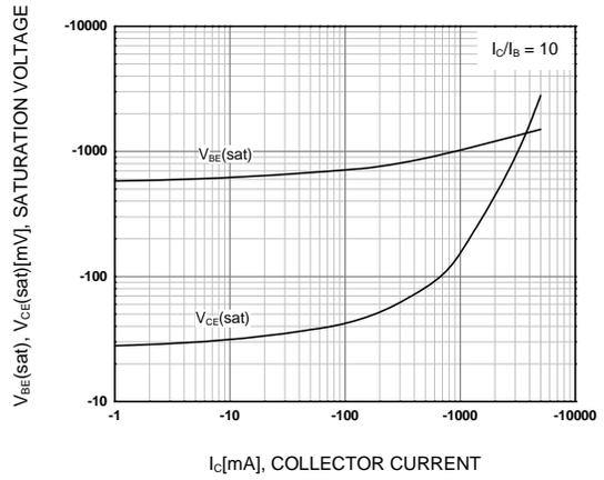
Figure 2. Base-Emitter Saturation Voltage and Collector-Emitter Saturation Voltage
