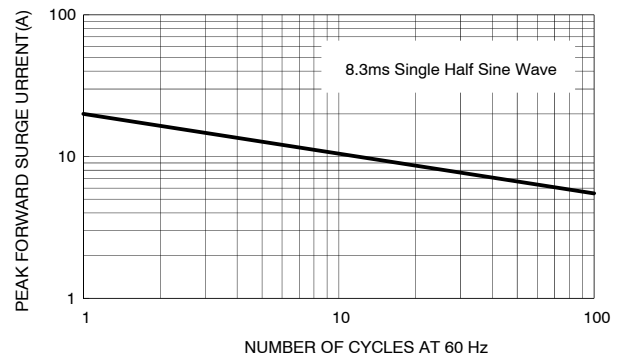
Figure 2. Maximum Non-Repetitive Forward Surge Current
