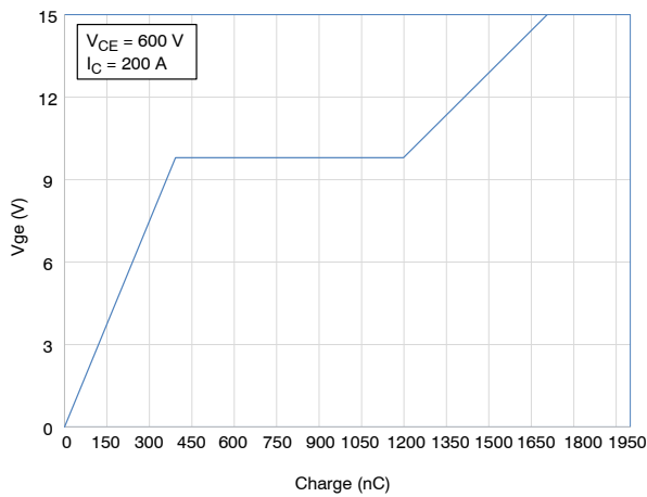
Figure 24. Gate Voltage vs. Gate Charge
