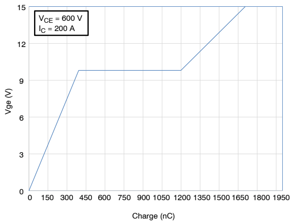
Figure 24. Gate Voltage vs. Gate Charge
