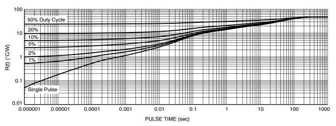
Figure 13. Thermal Characteristics
