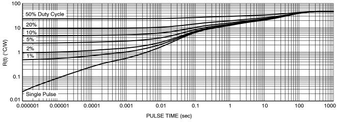
Figure 13. Thermal Characteristics
