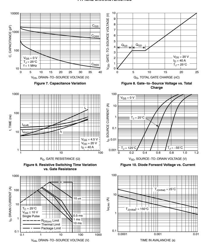
Figure 12. I<sub>PEAK</sub> vs. Time in Avalanche
