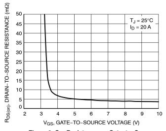
Figure 3. On-Resistance vs. Gate-to-Source Voltage
