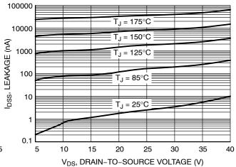
Figure 6. Drain-to-Source Leakage Current vs. Voltage
