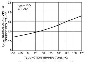
Figure 5. On–Resistance Variation with Temperature
