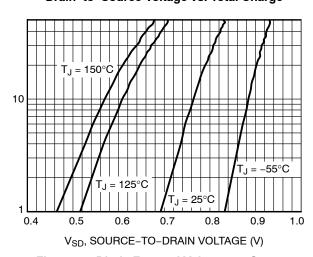
Figure 10. Diode Forward Voltage vs. Current
