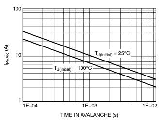
Figure 12. I<sub>PEAK</sub> vs. Time in Avalanche
