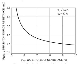
Figure 3. On-Resistance vs. Gate-to-Source Voltage
