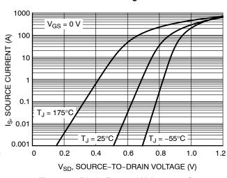
Figure 10. Diode Forward Voltage vs. Current
