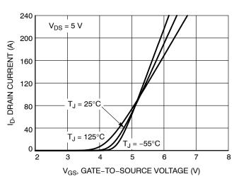
Figure 2. Transfer Characteristics
