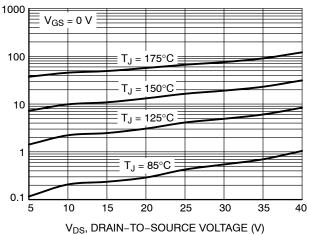
Figure 6. Drain-to-Source Leakage Current vs. Voltage
