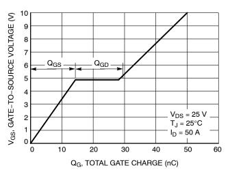
Figure 8. Gate-to-Source Voltage vs. Total Charge
