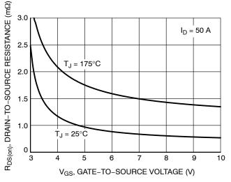
Figure 3. On-Resistance vs. Gate-to-Source Voltage
