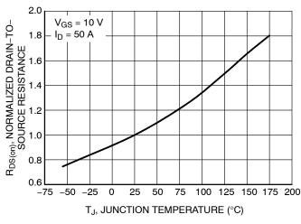
Figure 5. On–Resistance Variation with Temperature
