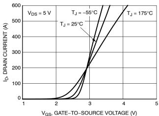
Figure 2. Transfer Characteristics
