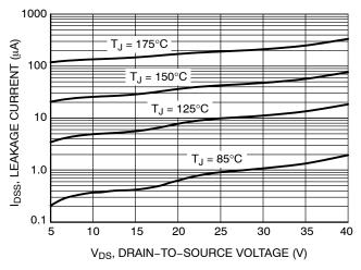
Figure 6. Drain-to-Source Leakage Current vs. Voltage
