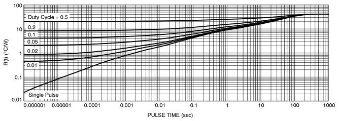
Figure 13. Transient Thermal Impedance
