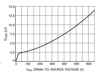
Figure 12. E<sub>OSS</sub> vs. Drain-to-Source Voltage
