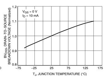
Figure 8. Breakdown Voltage Variation vs. Temperature
