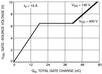
Figure 7. Gate Charge Characteristics
