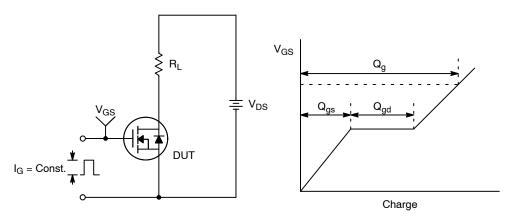
Figure 17. Gate Charge Test Circuit & Waveform
