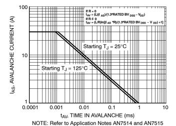
Figure 15. Unclamped Inductive Switching Capability
