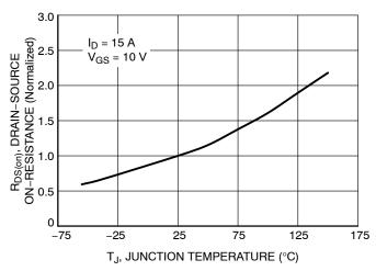
Figure 9. On-Resistance Variation vs. Temperature
