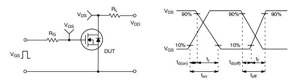
Figure 18. Resistive Switching Test Circuit & Waveforms
