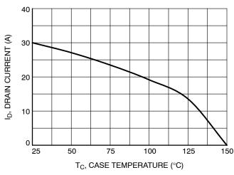
Figure 11. Maximum Drain Current vs. Case Temperature
