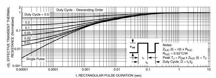
Figure 16. Transient Thermal Response
