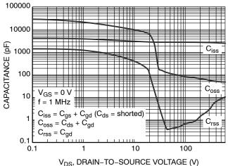
Figure 6. Capacitance Characteristics
