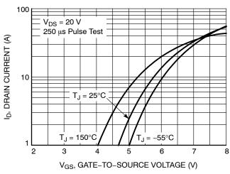
Figure 3. Transfer Characteristics
