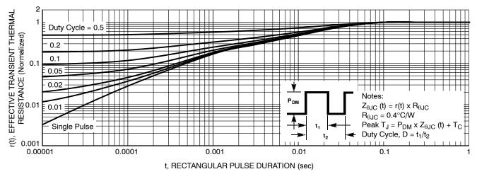
Figure 16. Transient Thermal Response
