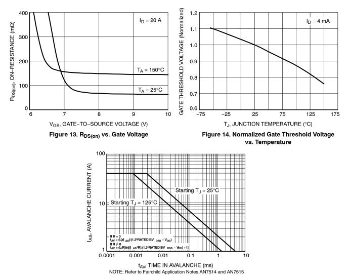
Figure 15. Unclamped Inductive Switching Capability
