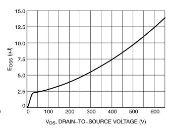
Figure 12. E<sub>OSS</sub> vs. Drain-to-Source Voltage
