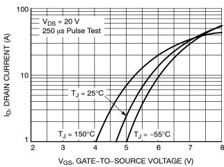
Figure 3. Transfer Characteristics
