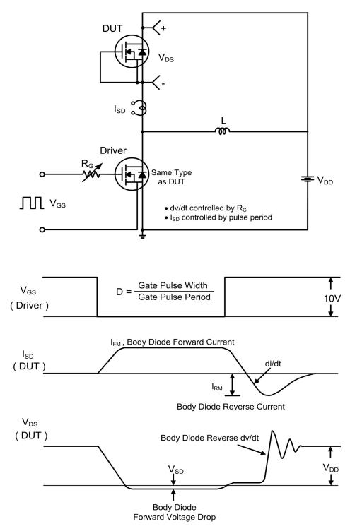
Figure 20. Peak Diode Recovery dv/dt Test Circuit & Waveforms
