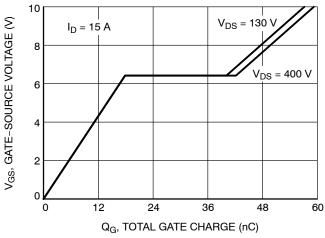
Figure 7. Gate Charge Characteristics
