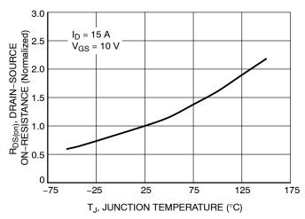
Figure 9. On-Resistance Variation vs. Temperature
