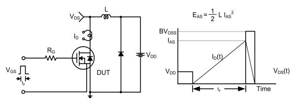
Figure 19. Unclamped Inductive Switching Test Circuit & Waveforms
