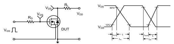
Figure 18. Resistive Switching Test Circuit & Waveforms
