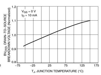
Figure 8. Breakdown Voltage Variation vs.
