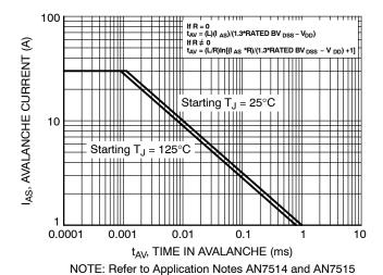
Figure 15. Unclamped Inductive Switching Capability
