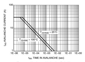
Figure 15. Unclamped Inductive Switching Capability
