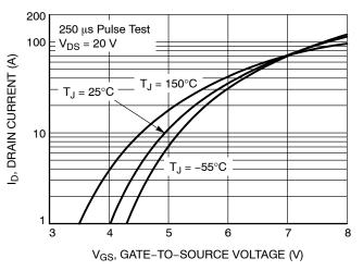
Figure 3. Transfer Characteristics
