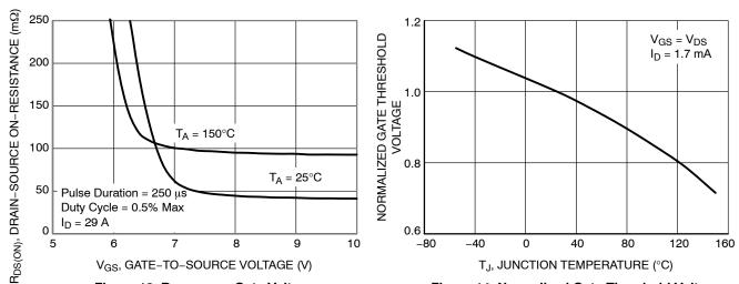
Figure 13. R<sub>DS(ON)</sub> vs. Gate Voltage
