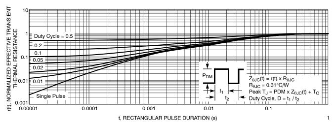
Figure 16. Transient Thermal Response Curve
