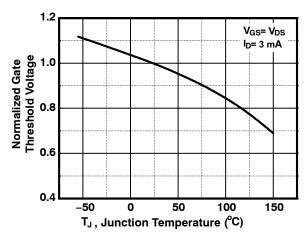
Figure 14. Normalized Gate Threshold Voltage vs. Temperature
