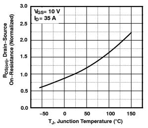
Figure 9. On-Resistance Variation vs. Temperature
