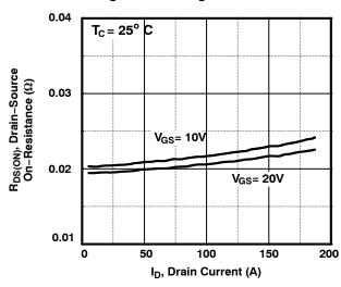
Figure 4. On-Resistance Variation vs. Drain Current and Gate Voltage
