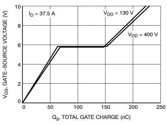
Figure 7. Gate Charge Characteristics
