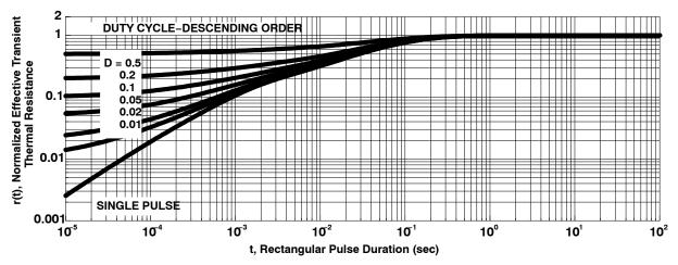
Figure 16. Transient Thermal Response Curve
