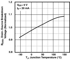
Figure 8. Breakdown Voltage Variation vs. Temperature
