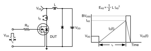
Figure 19. Unclamped Inductive Switching Test Circuit & Waveforms
