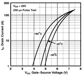
Figure 3. Transfer Characteristics
