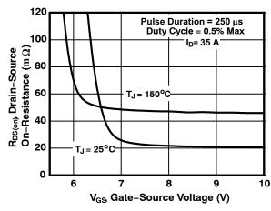
Figure 13. RDSON vs. Gate Voltage
