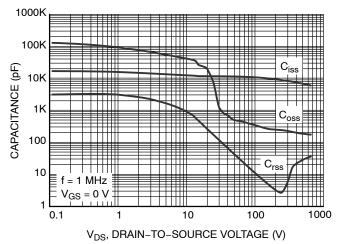
Figure 6. Capacitance Characteristics
