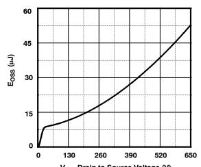
$V_{DS},$  Drain to Source Voltage (V) Figure 12. EOSS vs. Drain-to-Source Voltage
