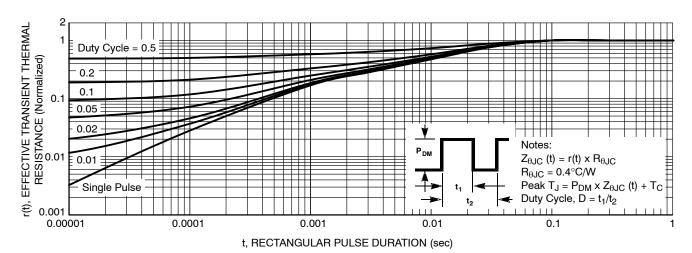
Figure 18. Transient Thermal Response
