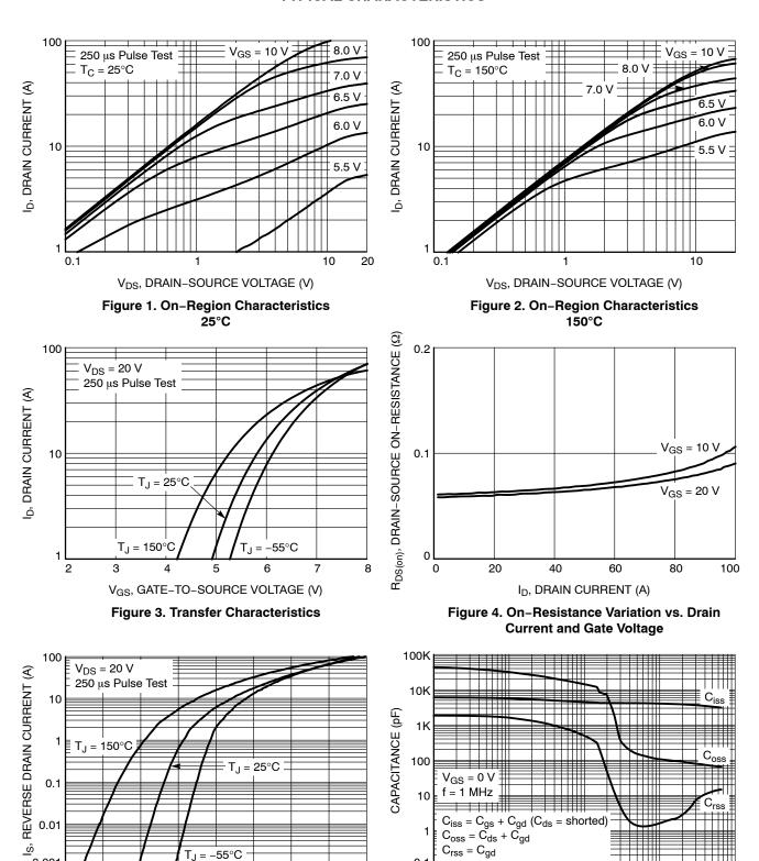
Figure 5. Body Diode Forward Voltage Variation vs. Source Current and Temperature
