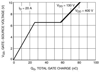
Figure 7. Gate Charge Characteristics
