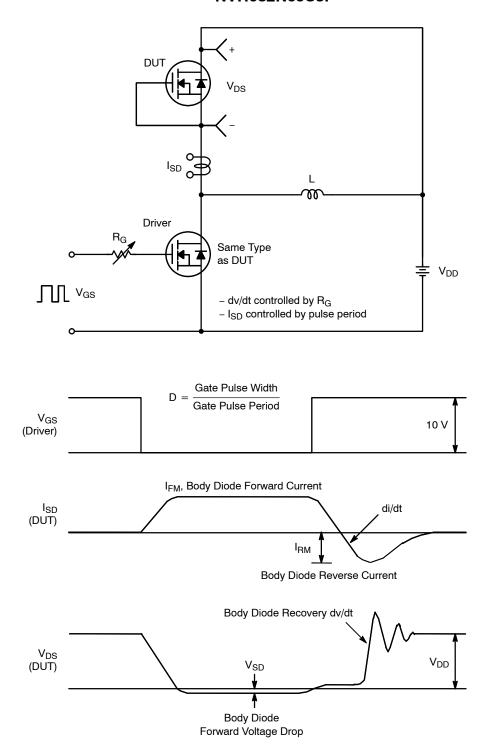
Figure 22. Peak Diode Recovery dv/dt Test Circuit & Waveforms
