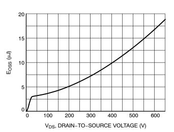
Figure 12. E<sub>OSS</sub> vs. Drain-to-Source Voltage
