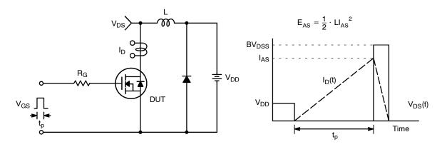
Figure 21. Unclamped Inductive Switching Test Circuit & Waveforms
