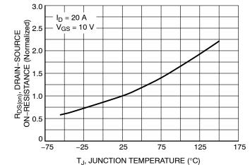
Figure 9. On-Resistance Variation vs. **Temperature**
