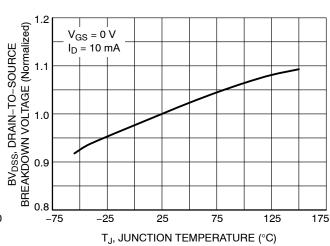
Figure 8. Breakdown Voltage Variation vs. Temperature
