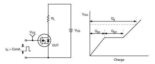
Figure 19. Gate Charge Test Circuit & Waveform
