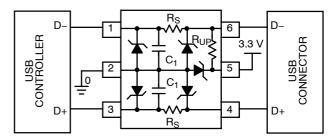
Figure 8. Low Speed Connection
