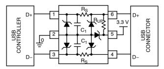
Figure 7. Full Speed Connection
