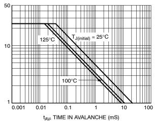
Figure 12. Maximum Drain Current vs. Time in Avalanche
