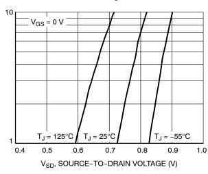
Figure 10. Diode Forward Voltage vs. Current
