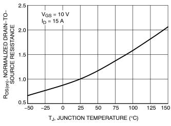
Figure 5. On-Resistance Variation with **Temperature**
