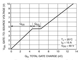
Figure 8. Gate-to-Source Voltage vs. Total Charge
