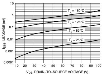
Figure 6. Drain-to-Source Leakage Current vs. Voltage
