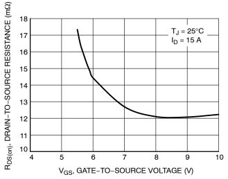
Figure 3. On-Resistance vs. Gate-to-Source Voltage
