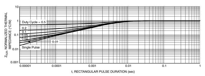
Figure 13. Transient Thermal Impedance
