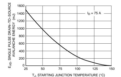
Figure 11. Maximum Avalanche Energy vs. Starting Junction Temperature
