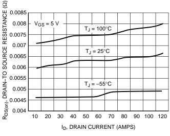
Figure 3. On-Resistance vs. Drain Current and **Temperature**
