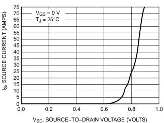
Figure 10. Diode Forward Voltage vs. Current
