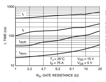
Figure 9. Resistive Switching Time Variation vs. Gate Resistance
