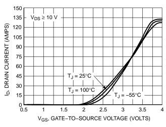
Figure 2. Transfer Characteristics
