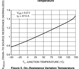
Figure 5. On-Resistance Variation Temperature
