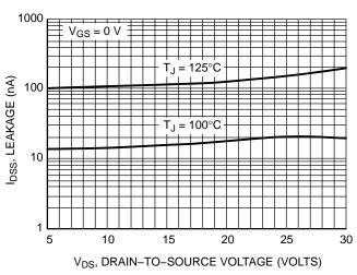
Figure 6. Drain-to-Source Leakage Current vs. Voltage
