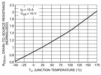
Figure 5. On–Resistance Variation with Temperature
