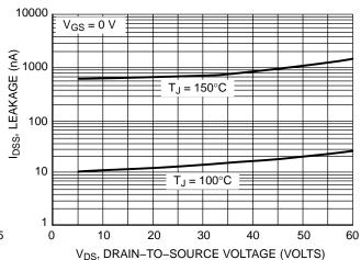
Figure 6. Drain-to-Source Leakage Current versus Voltage
