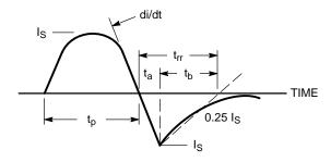
Figure 14. Diode Reverse Recovery Waveform
