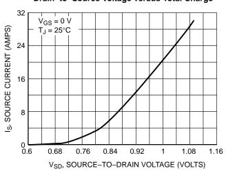
Figure 10. Diode Forward Voltage versus
