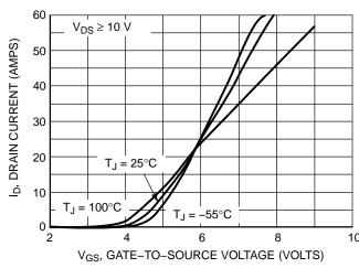
Figure 2. Transfer Characteristics
