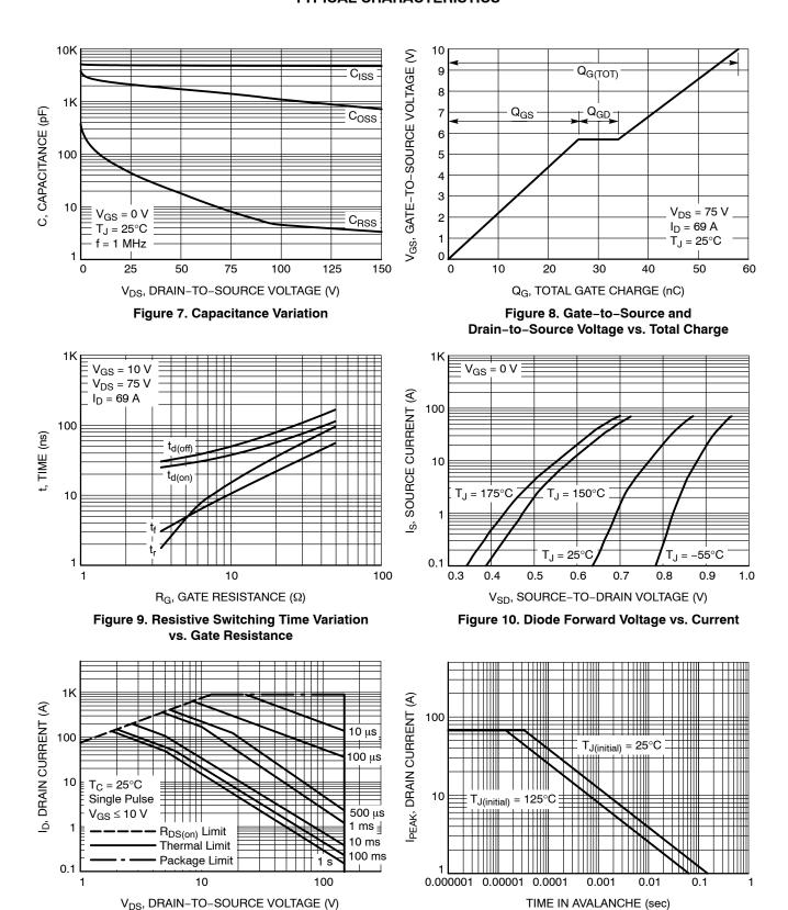
Figure 12. I<sub>PEAK</sub> vs. Time in Avalanche
