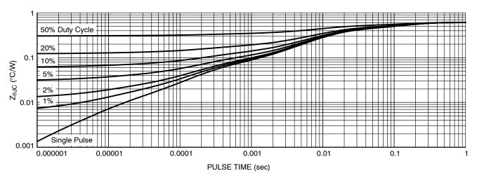
Figure 13. Thermal Characteristics
