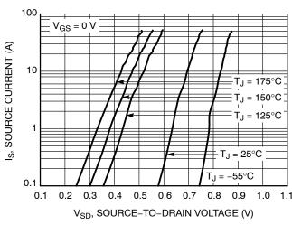
Figure 10. Diode Forward Voltage vs. Current
