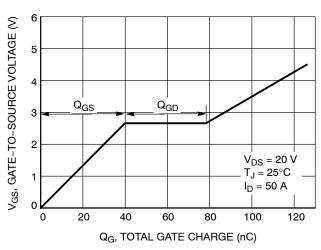
Figure 8. Gate-to-Source Voltage vs. Total Charge
