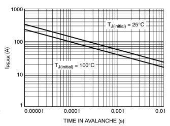
Figure 12. I<sub>PEAK</sub> vs. Time in Avalanche
