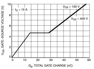
Figure 6. Gate Charge Characteristics
