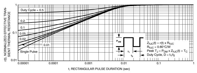
Figure 12. Transient Thermal Impedance
