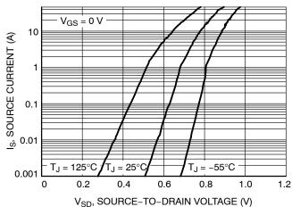
Figure 10. Diode Forward Voltage vs. Current
