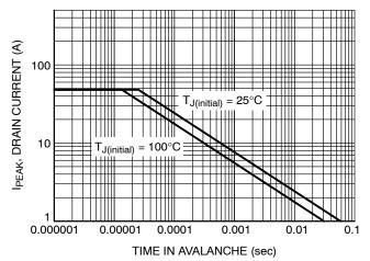
Figure 12. I<sub>PEAK</sub> vs. Time in Avalanche
