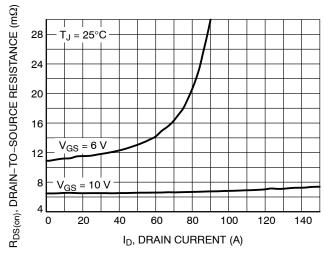
Figure 3. On-Resistance vs. Gate-to-Source Voltage
