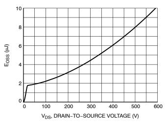
Figure 11. E<sub>OSS</sub> vs. Drain to Source Voltage
