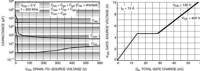
Figure 6. Gate Charge Characteristics
