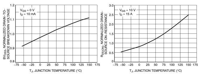
Figure 7. Breakdown Voltage Variation vs. Temperature
