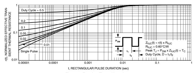
Figure 12. Transient Thermal Impedance
