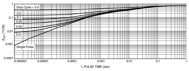
Figure 13. Transient Thermal Impedance
