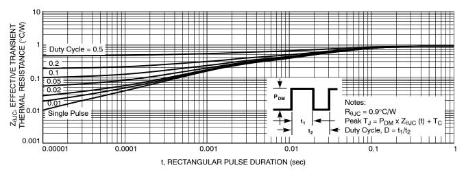
Figure 13. Transient Thermal Impedance
