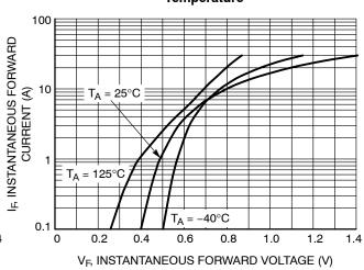
Figure 3. Typical Forward Characteristics
