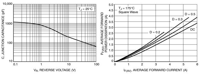
Figure 7. Typical Junction Capacitance
