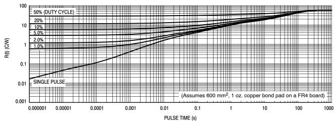
Figure 9. Typical Thermal Characteristics, Junction-to-Ambient
