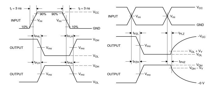
Figure 6. Switching Waveforms
