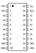
Figure 4. TSSOP Pinout (Top View)
