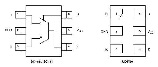
Figure 2. Pinout (Top View)
