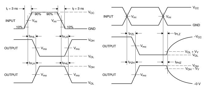
Figure 4. Switching Waveforms
